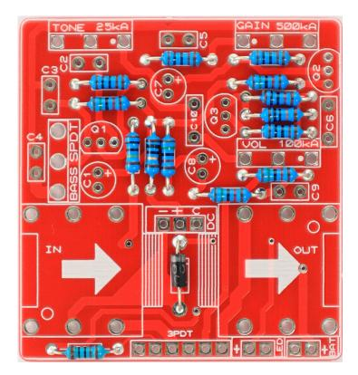
Place the resistors and diodes. If you have troubles reading the values, check out our <u>"Reading Part Values"</u> tutorial.
