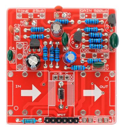
Solder the capacitors and transistors. If you have troubles reading the values, check out our <u>"Reading Part Values"</u> tutorial. Pay attention to the orientation, as well as to the polarity for electrolytic capacitors.
